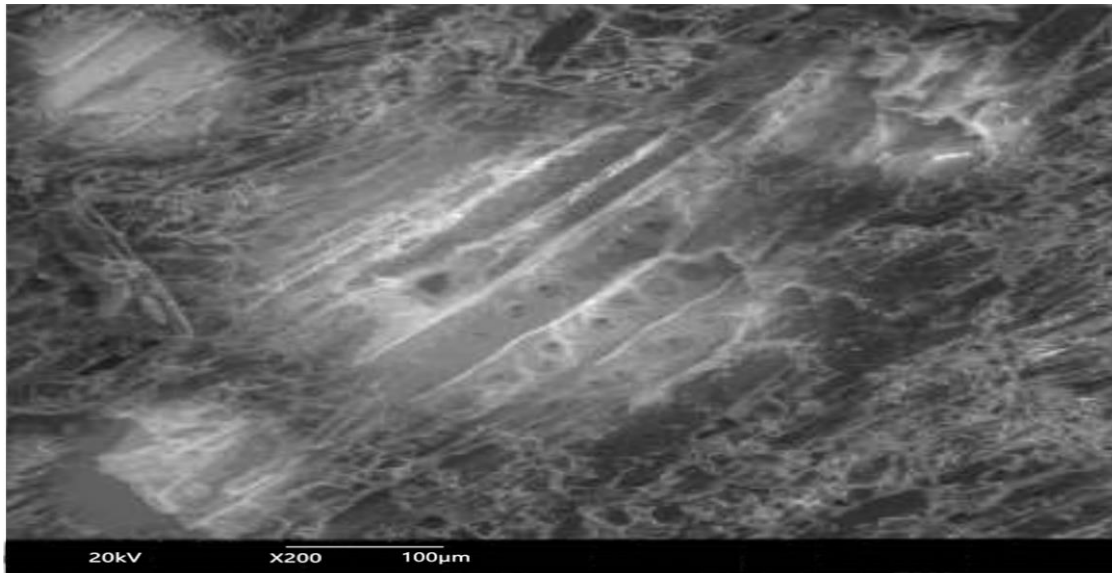
Figure 1: Scanning electron micrograph of Sawdust Activated Carbon (a) before and (b) after adsorption of dyes (Congo red and Tartrazine dyes).
